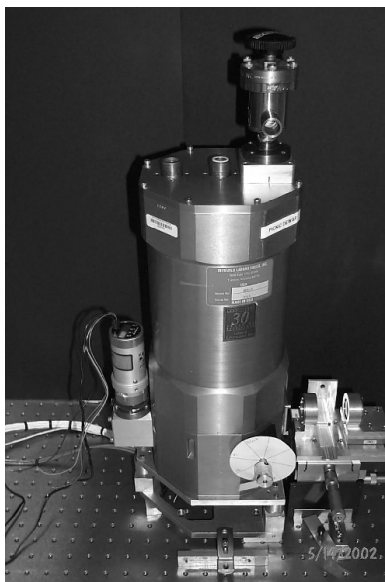
Figure 3. The PICNIC camera dewar and the optics focusing the beams from the IONIC3T beam combiner are shown in this picture. The mechanical assembly is an improved version of the previous NICMOS3 design, but the dewar is taller and contains more liquid nitrogen, one extra filter wheel is implemented, (in order to insert density filters), and both filter wheels are able to be motorised.
